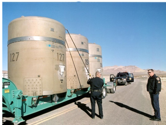
Figure 5. Highway Patrol Officers conduct radiological surveys on the first Nevada Test Site transuranic waste shipment at the Area 5 Radioactive Waste Management Complex located on the Nevada Test Site. These shipments travel on normal public roads to their final destination at the Waste Pilot Isolation Plant near Carlsbad, New Mexico. (source: NNSA)
